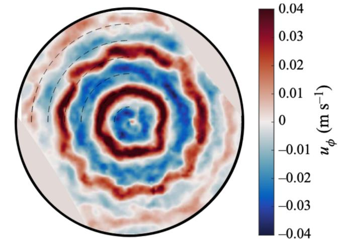
ZFs in rotating liquid column experiment Lemasquerier *et al* JFM 2021
