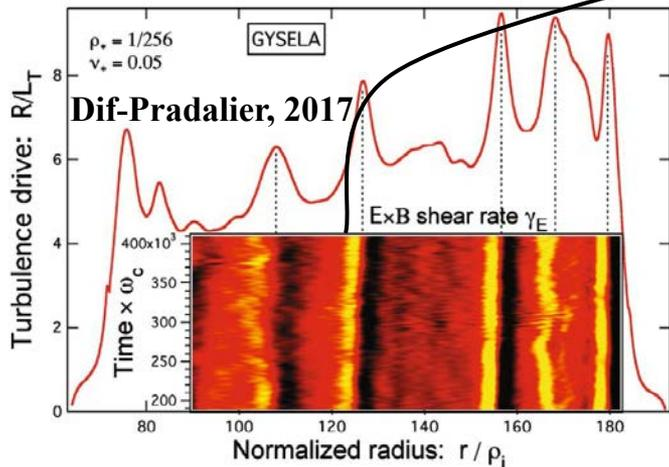
Yellow and black colors are a rapid transition of the direction of flows around peaks in turbulence drive.
