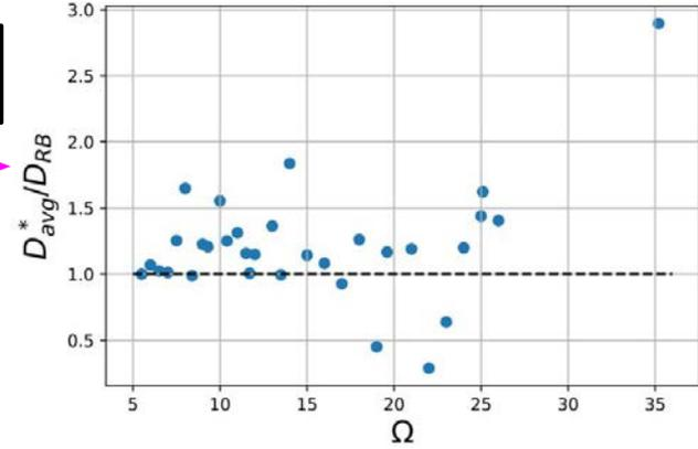
As cells fluctuate, the **effective diffusivity** deviates but **remains close** to the FCA effective diffusivity ( $D_{\text{RB}}$ ).
