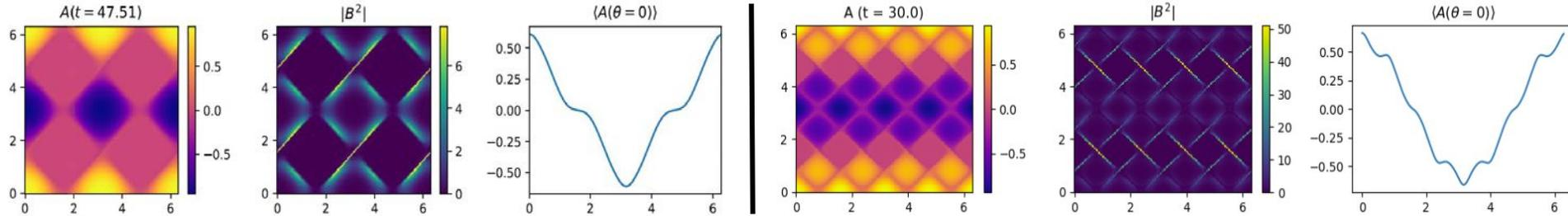
$A$  **homogenizes** within regions of **vortices**, thus producing **steps** in the profile. Magnetic field lines are expelled at boundaries and hold cell structure together.
