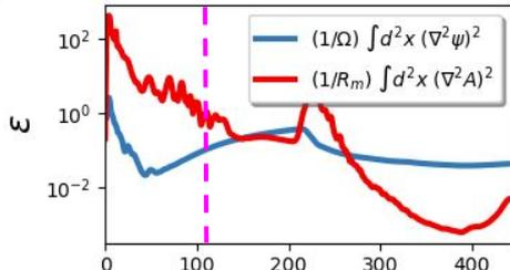
Cells wrap B-field during  $t < 100$  and flow enters a steady staircase state  $100 < t < 200$ . During flux expulsion magnetic energy dissipates at a rate greater than kinetic energy dissipation.
