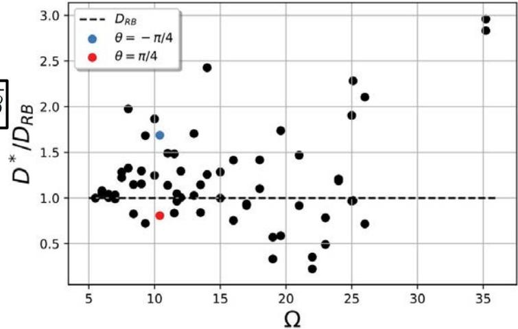
Effective diffusivity **increases/decreases** if the cells length along the gradient ( $d_x$ ) increases/decreases compared to the length perpendicular to the gradient ( $d_y$ ).
