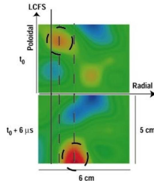
FIG. 4. (Color) Two frames from BES showing 2-D density plots. There is a time difference of  $6 \mu\text{s}$  between frames. Red indicates high density and blue low density. A structure, marked with a dashed circle and shown in both frames, features poloidal and radial motion.
