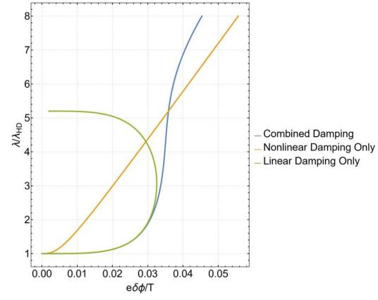
$\lambda/\lambda_{HD} \sim 3 \rightarrow 5$  for modest fluctuation levels at separatrix
