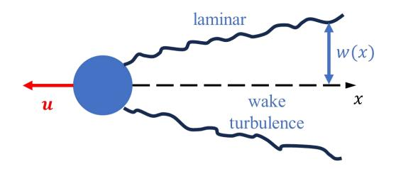
Turbulent wake, a simple, familiar example of spreading
