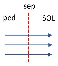
$\Gamma_0 \equiv$  turbulence energy flux at separatrix
