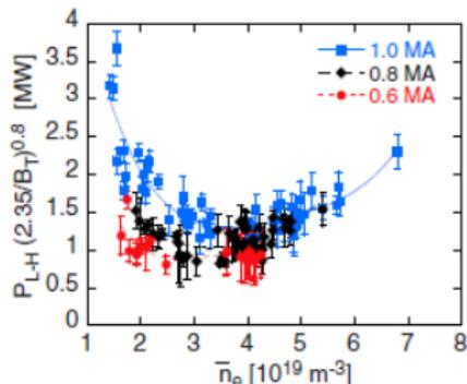
**Figure 3.** Power threshold versus density for the L–H transition normalized to  $|B_T| = 2.35$  T by the  $B_T^{0.8}$  dependence. The fits to the  $P_{L-H}$  data indicated here are also shown in figure 4. The error bars include all the contributions to  $P_{\text{tot}}$ . The larger error bars are due to the  $dW/dt$  term for discharges with a rather strong change of heating power before the occurrence of the L–H transition.
