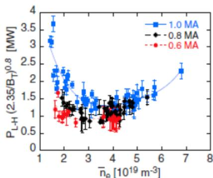
**Figure 3.** Power threshold versus density for the L-H transition normalized to  $|B_T| = 2.35$  T by the  $B_T^{0.8}$  dependence. The fits to the  $P_{L-H}$  data indicated here are also shown in figure 4. The error bars include all the contributions to  $P_{\text{loss}}$ . The larger error bars are due to the  $dW/dt$  term for discharges with a rather strong change of heating power before the occurrence of the L-H transition.
